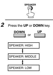
**3** When the display shows the desired volume level, press the **SPEAKER** key to turn off the speaker.
